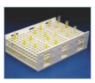
storage of samples. Steam autoclavable at 121°C (250°F). Per each, 6 per case.
