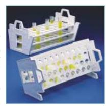
still hot, tilt the rack to the desired angle and allow media to harden. Rack may be used for incubating tissue cultures or submersed in a water bath. 40 places, numbered and lettered, for 16mm tubes. Not stackable. Polypropylene rack measures 267 x 152 x 130 mm H(10½ x 6 x 5½"H). Per each, 4 per case.
